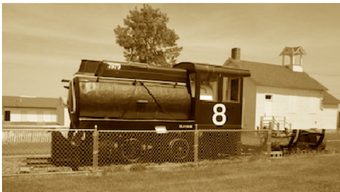
Dinky engine used to handle ties at the Tie Plant, now located at the fairgrounds. Courtesy of Crow Wing County Historical Society
